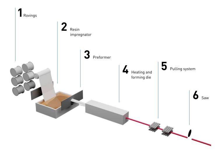
For around 70 years, the pultrusion process has been considered the process for manufacturing fiber-reinforced thermosets. Today, users have an almost infinite number of possibilities to produce the exact profile that perfectly fits their application. Perfect in terms of dimensions, structure and surface.
